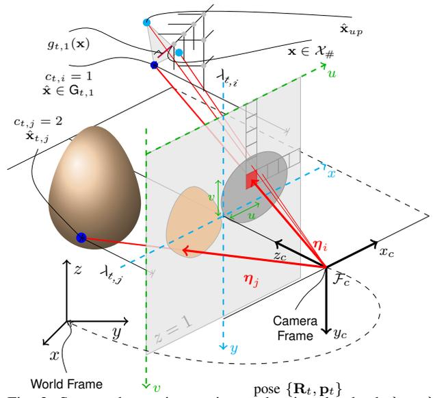
Fig. 2: Sensor observation at time  $t$  showing the depth  $\lambda_{t,i}$ ,  $\lambda_{t,j}$  and class  $c_{t,i}$ ,  $c_{t,j}$  measurements obtained along sensors rays  $\eta_i$ ,  $\eta_j \in \mathbf{E}$  when the sensor is at position  $\mathbf{p}_t$  with orientation  $\mathbf{R}_t$ . The inducing points  $\mathcal{X}_\#$  (c.f. Sec. IV-A) close to the observed surface are shown in gray.
